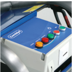
Control Panel (IP65) with Hourmeter
