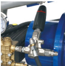
Hand adjustable Pressure Regulator [150 500 bar]
